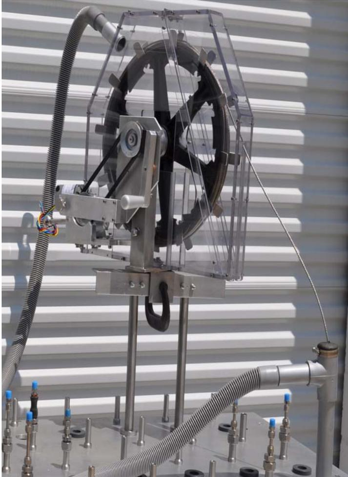
The redesigned hood arrangement allows for the front to completely open up via a top hinge, enabling open access to the reel and the eddy current cable and probe.
